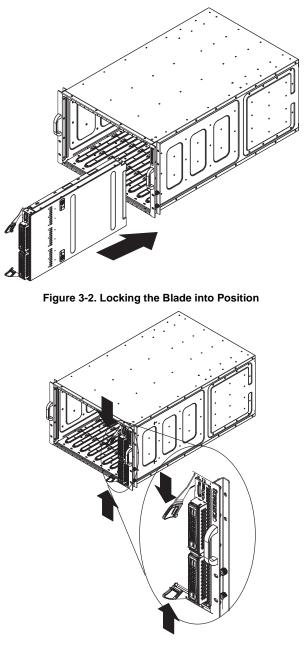
Figure 3-1. Inserting a Blade into the Enclosure
