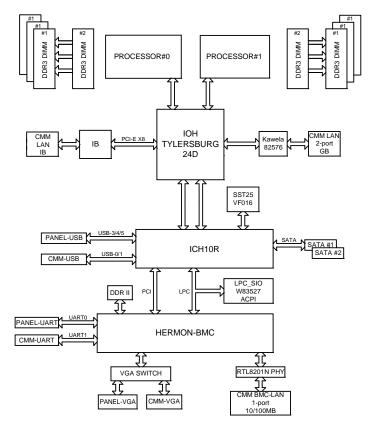
Figure 4-4. Intel 5500/IOH-24D Tylersburg + ICH10R Chipset: Block Diagram for SBI-7226T-T2
