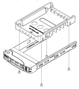
Figure 3-7. Installing a Hard Drive in a Carrier
