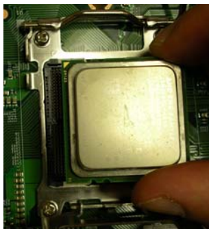
Figure 2-2. Aligning the CPU with Socket
