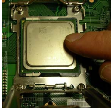
Figure 2-3. Placing the CPU into the Socket
