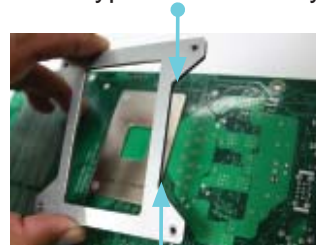
Install a Heatsink Bracket on the reverse side of the board
