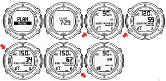
WHEN ENTERING THE PLAN MODE THE DISPLAY FIRST BRIEFLY SHOWS THE REMAINING DESATURATION TIME BEFORE GOING INTO PLAN MODE. USE UP AND DOWN BUTTONS TO SCROLL NO-DECOMPRESSION LIMITS AT DIFFERENT DEPTHS. YOU CAN ALSO ADJUST YOUR SURFACE INTERVAL TIME TO YOUR PLAN. NO-DECOMPRESSION LIMITS LONGER THAN 99 MINUTES ARE DISPLAYED AS "-"."
