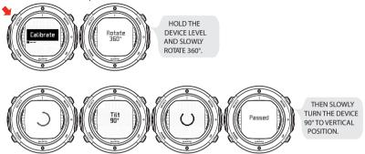
If the calibration fails several times in a row, it is possible that you are in an area with sources of magnetism, such as large metal objects, power lines or electric appliances. Move to another location and try to calibrate the compass again. If the calibration continues to fail, contact an authorized Suunto service center.
