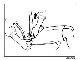
To unfasten the belt, push the red "PRESS" button on the buckle and allow the belt to retract.
