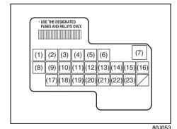
MAIN FUSE / PRIMARY FUSE (1) 15A Rear wiper (2) 15A Ignition coil (3) 10A Back-up light (4) 10A Meter (5) 15A Accessorv (6)15A Accessory 2 30A Power window (7)(8) 30A Wiper (9) 10A IG1 SIG (10)15A Air bag (11)10A Anti-lock brake system 4WD (12)15A 15A (13)Stop light (14)20A Door lock (15)Blank 10A ST SIG (16)(17)15A Seat heater (18)10A IG 2 SIG (19)10A Tail light (20)15A Dome
