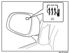
If the driver's outside rearview mirror has the mark (2), it is also equipped with the heated outside rearview mirrors. When you push the switch (1), both the heated outside rearview mirrors and the heated rear window will operate simultaneously.
