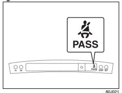
When the driver and front passenger don't buckle their seat belts, the driver's seat belt reminder light in the instrument cluster and the front passenger's seat belt reminder light in the information display will come on and a buzzer will sound as a reminder to the driver and front passenger to buckle their seat belts.
