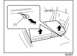
5) Pull the lock release strap (1) rearward to unlatch the seat cushion.
