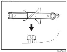
To stow the jack, place it in the storage bracket and turn the shaft clockwise until the jack is securely held in place.
