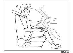
When seated as shown in the above illustration, the front passenger sensing system senses a properly-seated occupant and enables the air bag.
