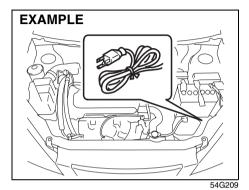
The engine block heater will help you start the engine more easily in very cold weather ( $-18^{\circ}$ C ( $0^{\circ}$ F) or below). To use the engine block heater:
