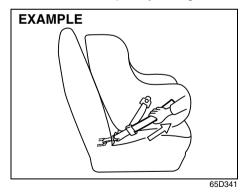
4) Return the seatback to the normal, upright position. Tighten the lower straps as described in the child restraint
