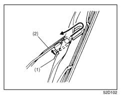
2) Squeeze lock lever (1) towards wiper arm (2) and remove the wiper frame from the arm as shown.
