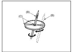
New discs may have some roughness around the edges. The unit may not work or the sound may skip if such discs are used. Use a ball-point pen (B), etc. to remove the roughness (C) from edges of the disc before insertion inside the unit.
