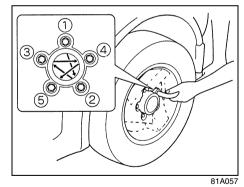
Wheel tightening torque
