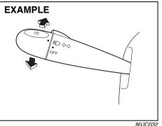
With the headlights on, push the lever forward to switch to the high beams (main beams) or pull the lever toward you to switch to the low beams. When the high beams (main beams) are on, a light on the instrument panel will come on. To momentarily activate the high beams (main beams) as a passing signal, pull the lever slightly toward you and release it when you have completed the signal.
