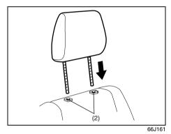
To reinstall the head restraint, insert the head restraint bars into the holes (2) and push the head restraint down.
