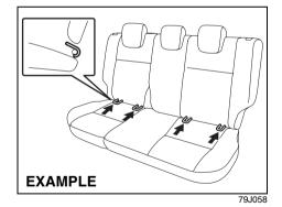
Your vehicle is equipped with lower anchors for securing up to one or two standard LATCH-type child restraint(s) in the second row seats. (LATCH stands for
