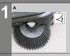
A Check the sweeping roller and the side brush for wear and wrapped belts.
