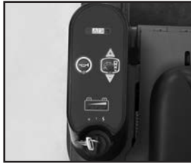
Simple one button control panel.
