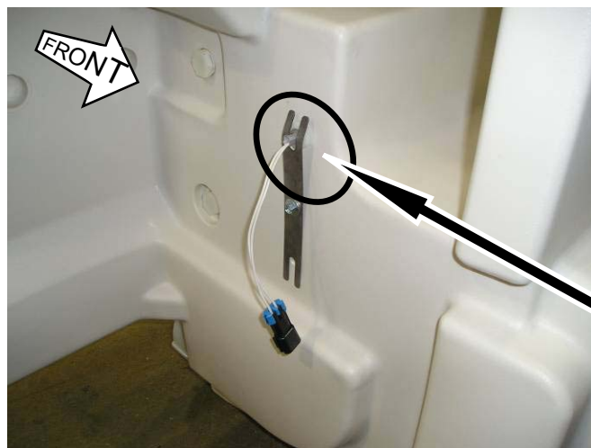
SOLUTION TANK FULL FLOAT SWITCH S9
