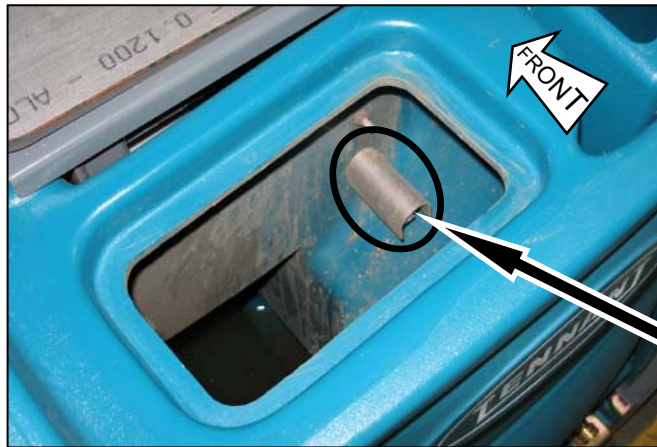
RECOVERY TANK FULL FLOAT SWITCH S4
