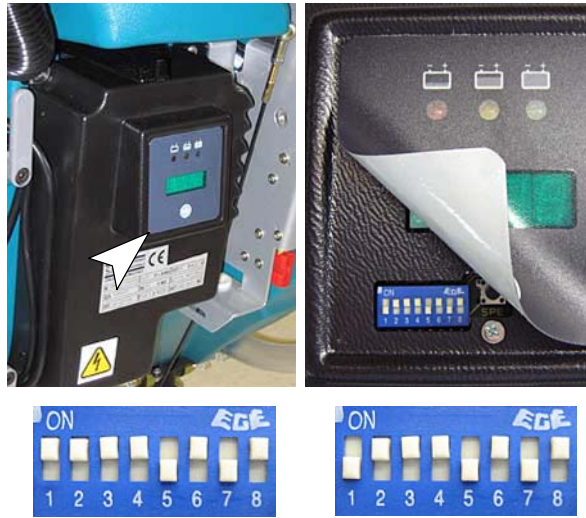
SEALED "GEL" BATTERY WET "Acid" BATTERY FIG. 42
