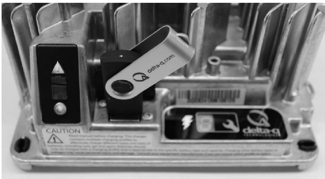
Figure 4, Insert the USB flash drive to begin the reprogramming process. When complete, the Fault/Error/USB Indicator will be solid green as shown.
