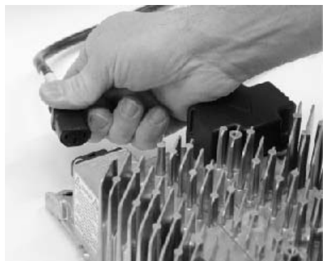
Figure 1: Disconnect AC input from the charger.
