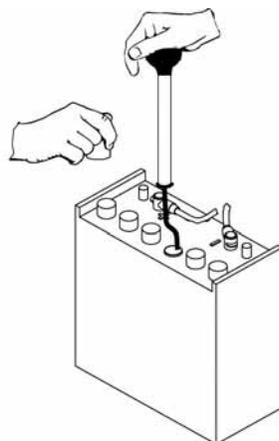
*NOTE: Do not take readings immediately after adding distilled water, if the water and acid are not thoroughly mixed, the reading may not be accurate.*
