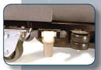
Externally mounted solution filter
