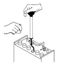
NOTE: Do not take readings immediately after adding distilled water, if the water and acid are not thoroughly mixed, the reading may not be accurate.
