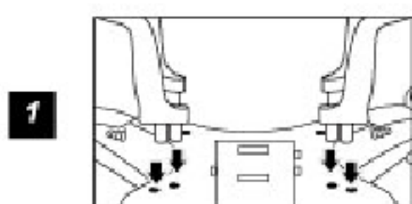
1. Install the landing gear to the bottom of drone and tighten screws
