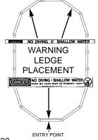
Your pool is equipped with (3) three special **warning** ledges. The (1) one ledge with a large **warning** on top is to be installed by the entry point into the pool and is not to be obstructed by any object such as your ladder. The (2) two ledges with the **warning** on the inside are to be placed opposite the entry point into the pool with the warning facing the entry point.
