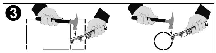
If the through wall filter inlet and outlet holes are to be used, remove metal cutouts by breaking perforations using a knife and hammer as shown. Refer to skimmer manufacturer's instructions for remainder of skimmer assembly. Make sure skimmer does not leak as this will corrode the pool wall and cause a split in the wall that is not covered under the pool warranty.
