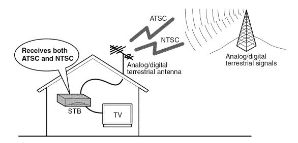
Digital broadcasting is the most advanced format of broadcasting, employing a new technology for compression of audio and video signals which allows broadcasters to transmit digital signals using existing terrestrial systems.
