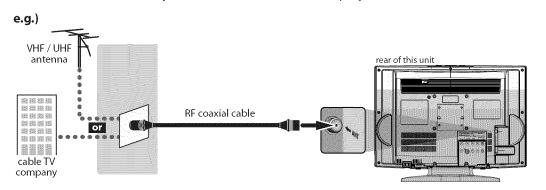
\*Once connections are completed, turn on the unit and begin initial setup. Channel scanning is necessary for the unit to memorize all available channels in your area. (Refer to "Initial Setup" on page 12.)
