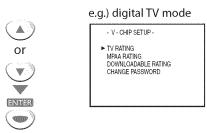
Use [Cursor ▲/▼] to select the desired rating, then press [ENTER] repeatedly to switch between "VIEW" and "BLOCK".
