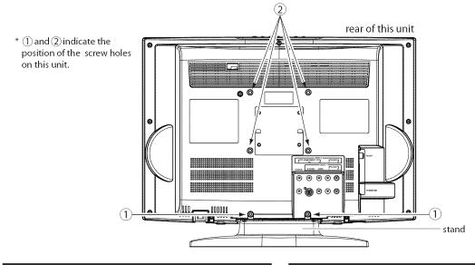
Turn this unit over and place it screen-first onto a table which has a soft cloth draped over it.
