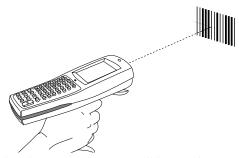
3. Ensure that the scan beam crosses all bars and spaces on the bar code symbol, as shown below:
