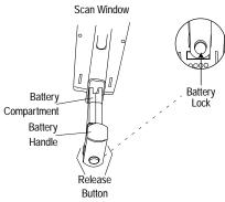
3. Press the battery lock in to secure.
