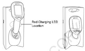
3. The mobile computer starts to charge automatically. The mobile computer fully charges in approximately five hours. While charging, a red charging LED can be seen through the front panel of the cradle behind the mobile computer. Refer to the MC17 Product Reference Guide for specific charging profile information.
