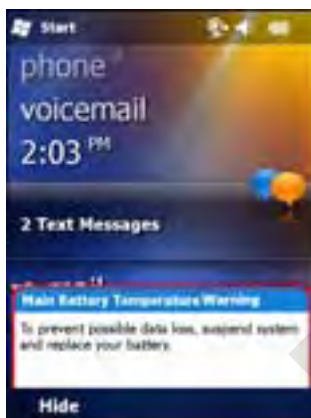
Figure 2-14 Main Battery Temperature Warning Dialog Box
