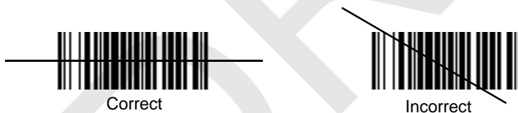
Figure 3-2 Linear Scanner Aiming Pattern
