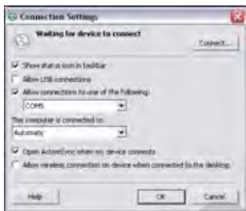
Figure 6-31 ActiveSync Connection Settings Window on PC
