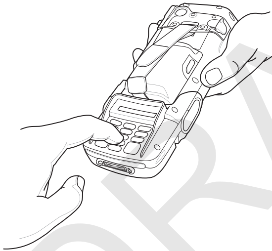
Figure 7-17 Enter PIN on DCR
