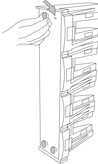
Figure 2-6. Installing Suction Cups on the CRD 38/6866
