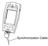
Plug the power cable into a wall outlet and plug the other end into the battery charging receptacle on the side of the synchronization cable.
