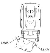
Insert the lithium-ion battery in the battery compartment with the battery tether positioned properly (as shown below), making sure the battery snaps into place.
