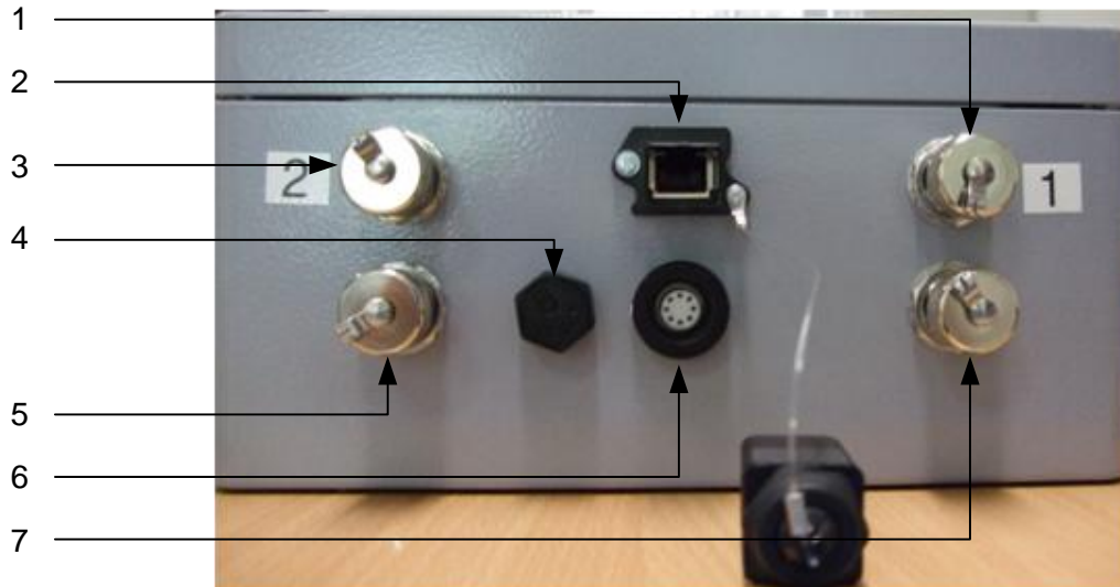
Figure 10 - interfaces of LPR station on a vehicle as double receiver
