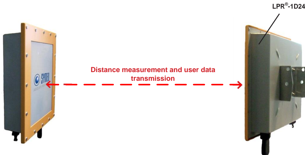
Figure 1: LPR®-1D24 measurement path
