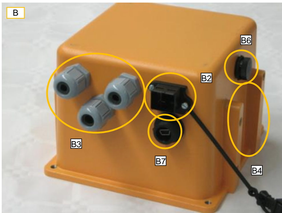
Figure 5: Rear element of the LPR-1DHP station
