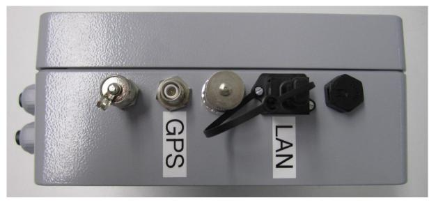
Attention: The STU is only rated IP65 if prober connectors (e.g. Harting Push Pull RJ45 part number 09451451100) are used and if all unused feed-through are properly sealed.
