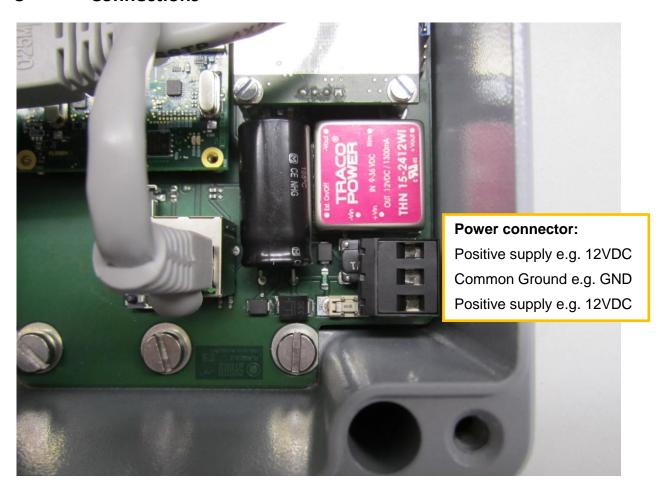
Power has to be connected to internal 3pin terminal connector. Ground has to be connected to the terminal 2 (terminal in the middle of the connector), positive DC supply can be connected to two outer terminals. The STU is fused, protected against overvoltage and against reverse polarity.
