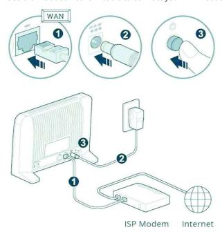
2 Connect one end of the power adapter to the power port on your MR2200ac, and the other end to the power outlet. Press the power button to power on your MR2200ac. Wait for around two minutes until the STATUS LED indicator starts blinking blue slowly.
