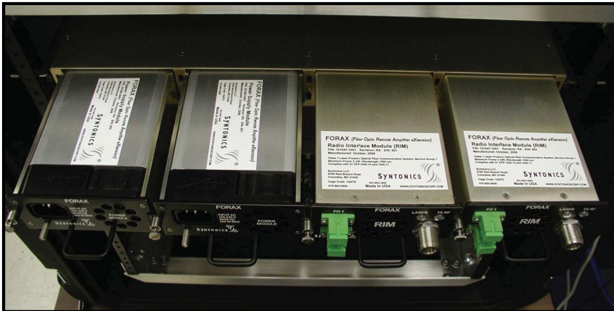
Figure 2-1. 1U OIU Chassis with All Modules Partially Inserted
