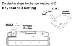
Warning!:The above steps shall be completed within 10 seconds. Otherwise, the ID connection might be failed and need to re-connected again.
