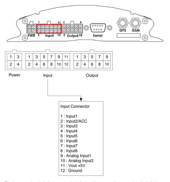
The Input number 1, 2, 3, 4 are positive triggered inputs and Input number 5, 6, 7, 8 are negative triggered inputs. If you would like to use power saving function, please connect the Input2/ACC to ACC wire. The analog inputs are reserved.
