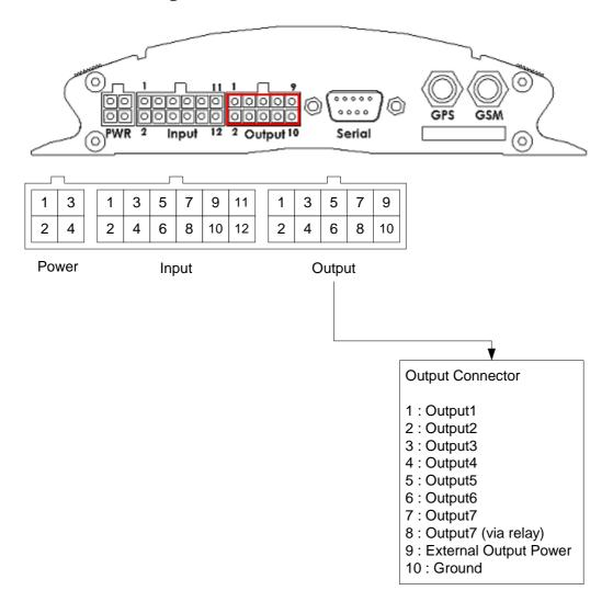
The output number 1, 2, 7 are positive triggered outputs and output number 3, 4, 5, 6 are negative triggered outputs. Pin number 7 and 8 are controlled by the same signal (OutputID = 7), Pin7 is positive trigger and pin8 is negative trigger. The OutputID = 8 is reserved for immobilizer control.
