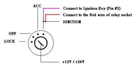
(3) For security reason, it is better do NOT install the wireless relay at IGNITION key lock area. May install the wireless relay in the hood or near the fuel pump or any confidential place for engine disable cutting.
