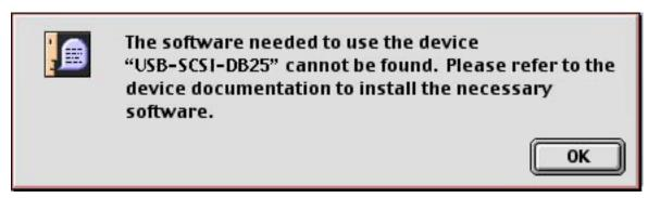
If this occurs, click "OK", install the driver software, and then attach the FireWire connector.
