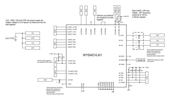
Note1: All IO pins should be left open (no need to pull-up or pull-down) if not used.
