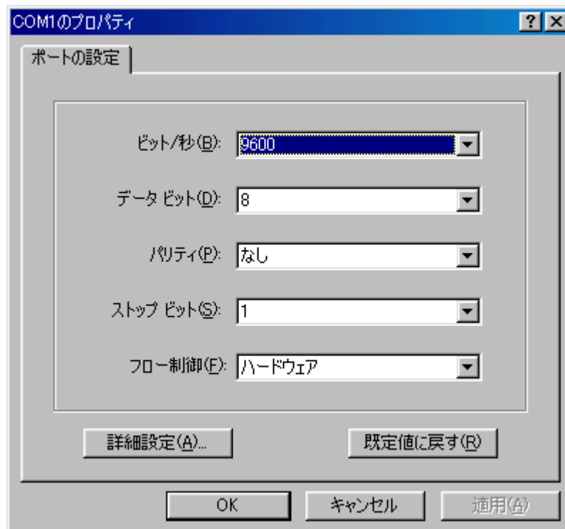
Fig.4-3-3 Setting window of COM PORT
