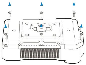
3 Remove the back of the camera.
