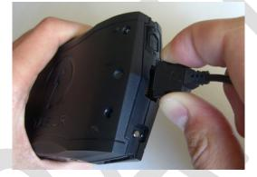
2. Connect the HeadCam cable to the ComHub. Make sure that the "diamond" on the connector is facing the back of the ComHub device.
