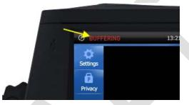
The **BUFFERING** mode is the default mode of operation, and is activated immediately after power-up and log in. During the Buffering mode, the touch screen operates similar to a viewfinder on a digital camera or video recorder. It provides real-time display of images based on the orientation of the HeadCam.
