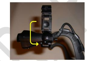
3. Thread the wire from the HeadCam through the cable management clips in the headband.
