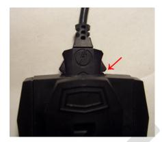
NOTE: It is important to make sure that the cable plugs have a good connection and that they are seated properly in their slots. Sometimes, it might look like they are secure when they actually are not, so make sure that the cable plug is seated all the way in.
