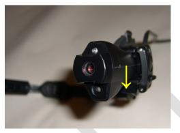
2. Close the imager clamp on the HeadCam. You should hear a snap when it shuts.
