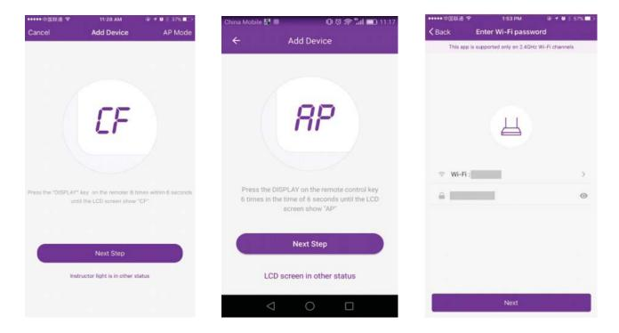
3. Select the AC Device as name "SmartLife-XXX" at the WLAN setting, then back to the APP interface. The APP will automatically do match.
