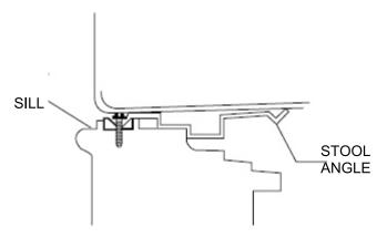
Fasten cabinet to window sill using two 7/8" Round -Head screws. Pre-drill holes if needed. Add the bottom rail seal over the screws.
