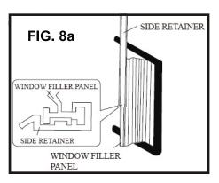
Insert top and bottom legs of window filler panel frame into channel in the top angle and bottom rail. Do both sides. Install side retainer to cabinet as shown. FIG 8B-
