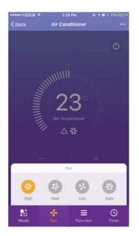
4. Other function control can by selected by "Function" button, Sleep, ECO. When Sleep mode, the fan speed will be fixed to low speed.
