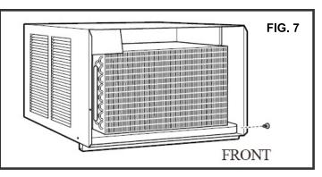
7. Hold the cabinet while pulling on the base handle to carefully remove the unit. Do not pull or lift near the top of the unit (FIG 8).
