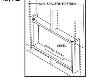
**NOTE**: If wall thickness is 8-1/2" or more, add aluminum flashing over the bottom of the frame opening to assure water is unable to enter the area between the inner and outer wall.
