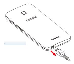
Unplug the AC adapter from the outlet, and remove the micro USB cable from the phone and the AC adapter.
