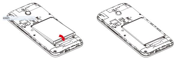
Align the contacts of the battery with the contacts in the phone.
