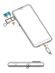
Caution: Do not insert the SIM pin into the microphone on top of the phone.
