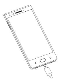
Connect the battery charger to your phone and power source respectively, the LED indicator will light while charging.
