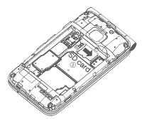
② To insert MicroSD card, push the MicroSD card into the card slot with the gold-colored contacts facing down.
