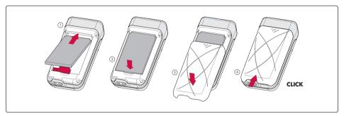
Insert and click the battery into place, then close the telephone cover.
