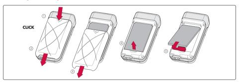
Unclip the cover, then the battery and remove it.
