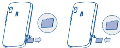
Unclip the back cover and insert the MicroSD card into the slot. Unclip the back cover and gently push the memory card until unlocked. Take out your MicroSD card and clip the back cover.
