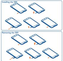
Insert the SIM card into the slot with the chip facing downwards until it is locked. To remove it, gently push the SIM card until it is unlocked.
