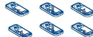
To release the MicroSD card holder, slide it in the direction of the arrow and lift it. Then insert the MicroSD card with the golden contact downward. Finally, turn down the MicroSD holder and slide it in the opposite direction to lock it.
