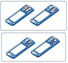
Insert the microSD card with the golden contacts facing downwards into the slot. To remove the microSD card, gently press and slide it out.
