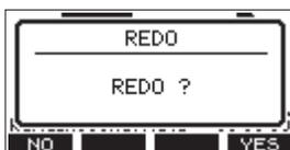
2. Press the **F4 YES** button to restore the previous operation and return to the state before undoing.
