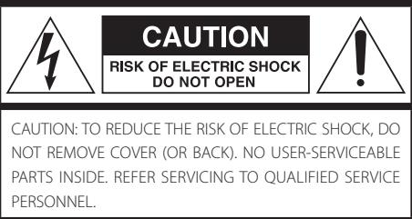
The lightning flash with arrowhead in an equilateral triangle is intended to alert the user to the presence of uninsulated "dangerous voltage" within the product's enclosure that could be of sufficient magnitude to constitute a risk of electric shock to persons.
